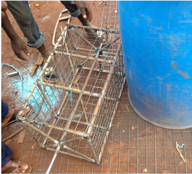
Figure 3: The local welders construct the improvised interior of the honey extractor
