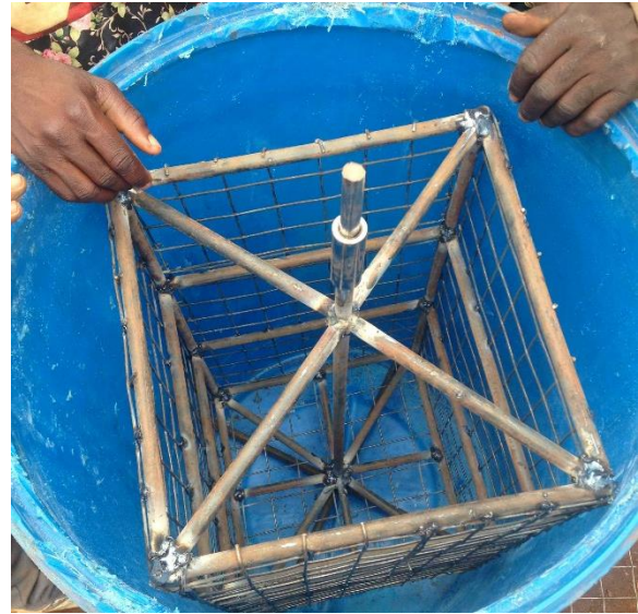
Figure 4: The interior of the honey extractor sits inside its plastic drum housing
